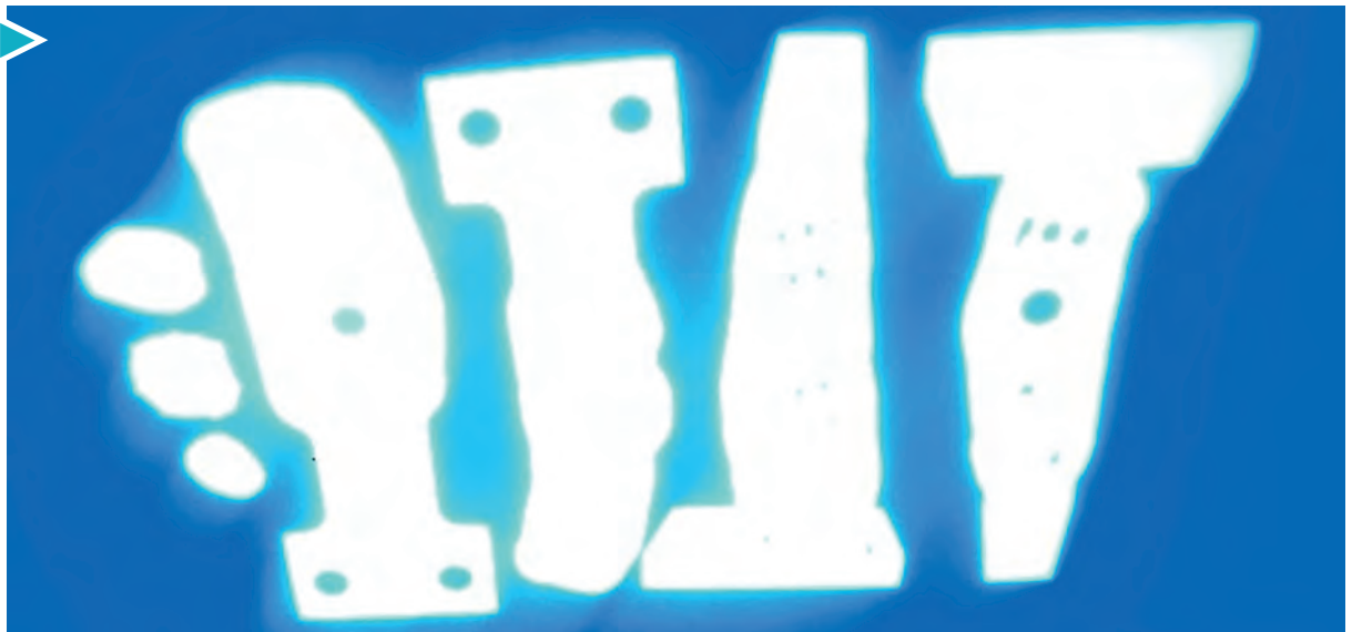
Fig. 2 DLP technology: light projection via LED
