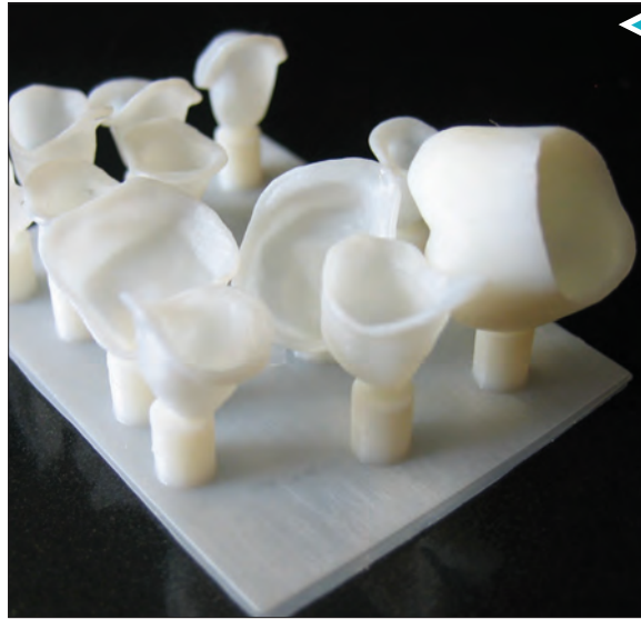
Fig. 6 Use of Detax resin for the printing of guides, rims, and temporaries of different shades.
