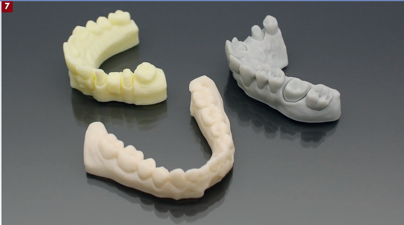
Models printed in Freeprint model material, ivory, sand and grey
